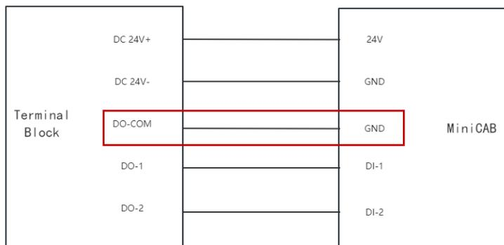
Figure 5.2 Terminal block and MiniCab wiring diagram
