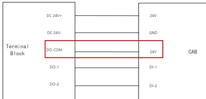
Figure 5.1 Terminal block and CAB wiring diagram
