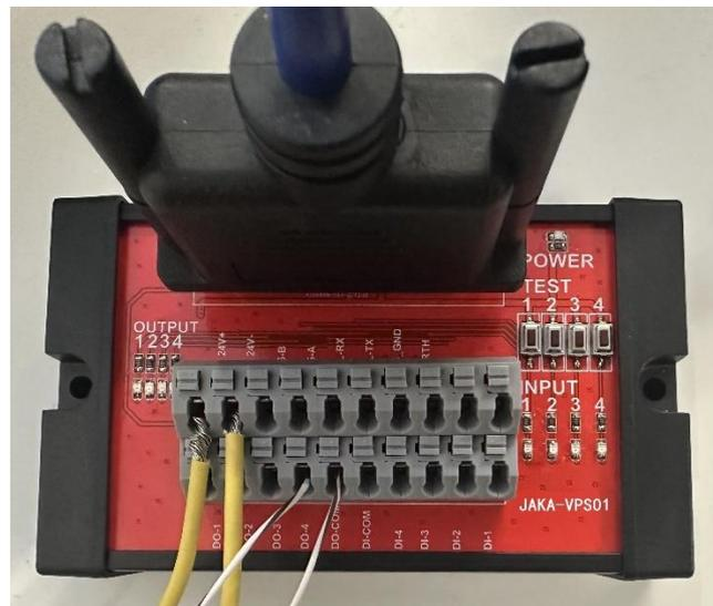
Figure 2.3 Terminal board wiring diagram
